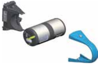
Figure 3: The intrinsically safe sensor head can be removed and replaced even while the transmitter is located in fully combustible hazardous atmospheres.
