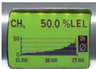
Figure 4: IR 29 transmitters are available with or without a built-in display. In the "Histogram" mode readings are displayed in the form of a constantly updated column chart, making it easy to visually evaluate changes and trends in the gas concentration.
