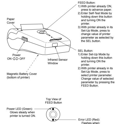
Figure 1. Component Locations and Functions
