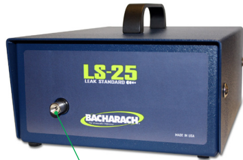
LS-25 Leak source
