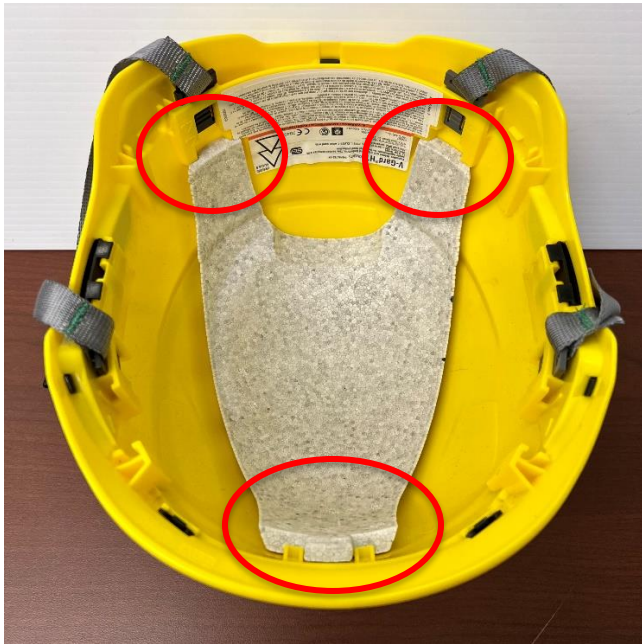
OLD Foam Liner (Does NOT meet EN12492 Clauses)
