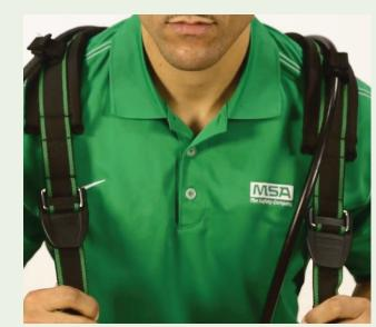
As you straighten up, pull shoulder strap tabs out. Hike unit up for a comfortable fit. Shoulder straps and waist-strap ends must be tucked in and lay flat across the body.
