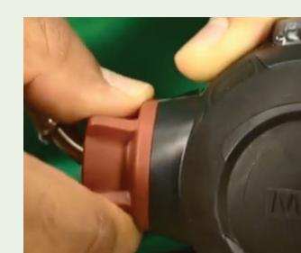
Crack bypass valve slowly to bleed off pressure until gauge needle drops below: 550 psig for 2216
