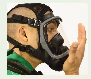
To check **facepiece fit**, hold palm of your hand over inlet connection and inhale. Hold our breath at least 10 seconds. The facepiece should collapse and stay collapsed against your face. If it does not, readjust facepiece and test again.
