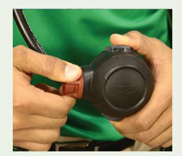
Grasp mask-mounted regulator and push top release buttons. Check that **red bypass knob** is fully closed (clockwise).
