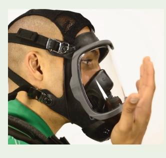
To test **exhalation valve**, take a deep breath and hold it. Block the inhalation connection with the palm of your hand and exhale. If exhalation valve is stuck, you may feel a heavy rush of air around the facepiece.
