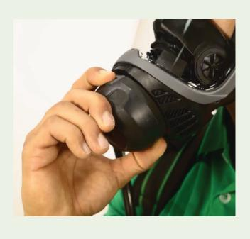
Push the **release buttons** and pull the regulator down and out of the facepiece adapter.
