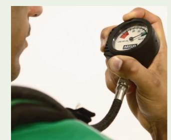
Close cylinder valve and watch **pressure gauge**. If needle drops more than 100 psig in 10 seconds, there is a leak. Do not use the apparatus until the leak is found and corrected.
