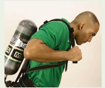
**Reach** inside right shoulder strap and grasp pressure gauge, slide left arm through left shoulder strap. **Bend** forward slightly, rest it on your back.
