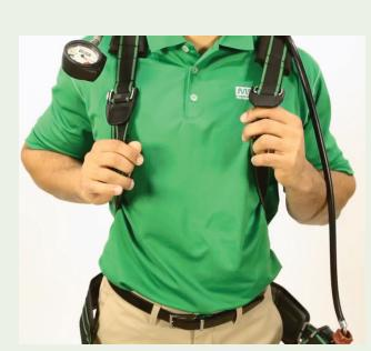
To **remove the facepiece**, fully loosen the harness straps and pull the facepiece up and away from your face. To remove the carrier harness, press the **belt buckle release buttons** IN. Disconnect chest strap (if used). To loosen the shoulder straps, grasp the release tabs. Push them out and away from your body. Slip your right arm out of the shoulder strap first, then remove the harness.
