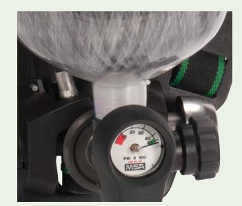
Check that cylinder is fully **pressurized**. Ensure that the Audilarm coupling nut is hand tight.
