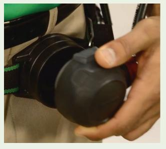
Close cylinder valve fully. Open bypass to **release system pressure**. Close bypass. Stow regulator with red bypass knob pointing to the right in STAND-BY belt mount.
